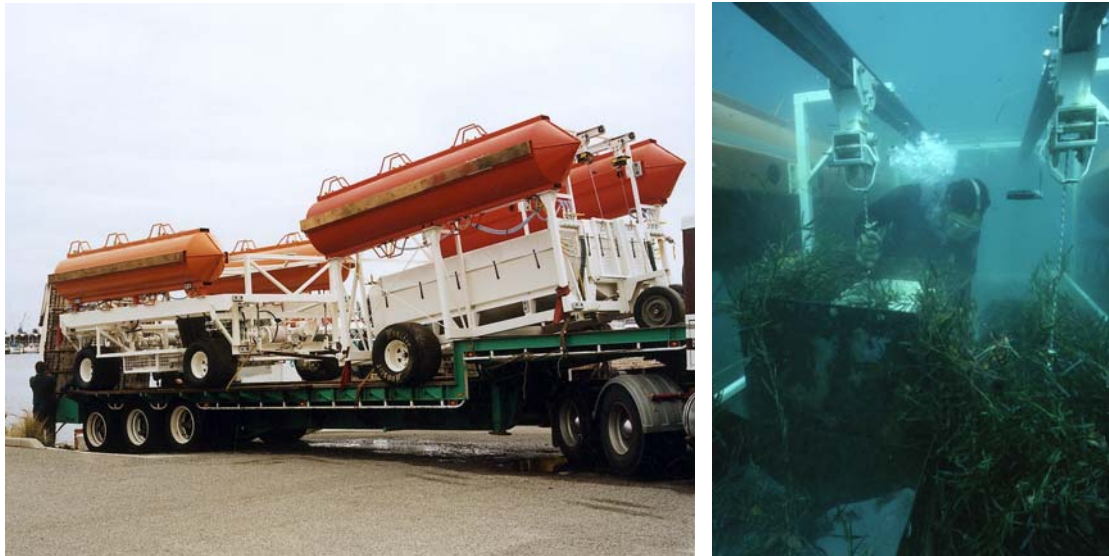
Figure 2. Photographs of ECOSUB1 on a trailer (left) and underwater collecting large cores of Amphibolis antarctica from a donor meadow (right) (Photographs from van Keulen and Paling, 2002).
