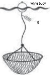
A **drop net** is made of two hoops that are joined by a cylindrical or cone shaped net bag. A maximum hoop diameter of 107 cm applies. Drop nets do not need to be registered but must be buoyed and tagged correctly, with a white buoy of 4L volume and a tag showing the owner's name and address.
