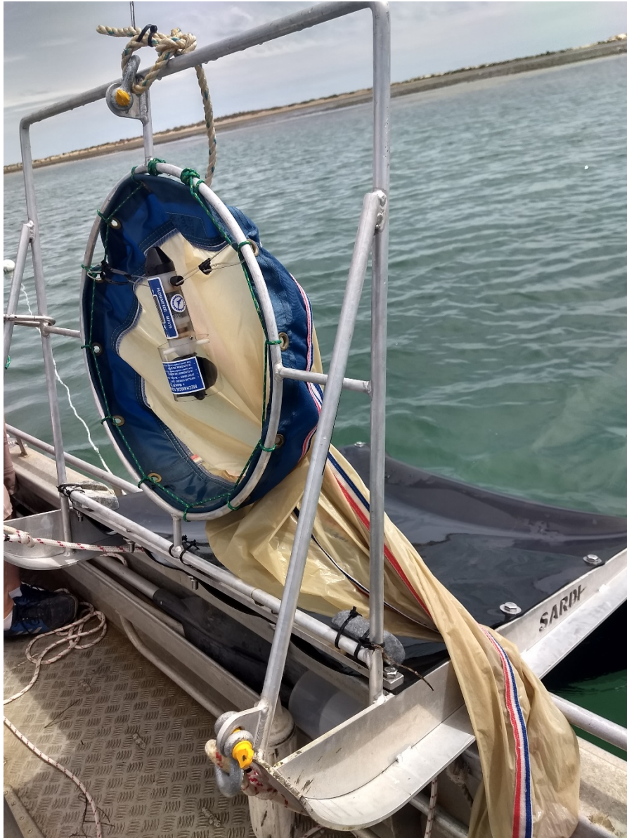
Figure 1. Plankton net mounted on benthic sled for collection of near-bottom plankton samples.
