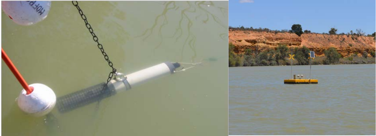
Figure 7. Loggers that are deployed in the Lower Murray River to measure dissolved oxygen concentrations (left) and the typical mooring station (right) (photos: University of Adelaide).
