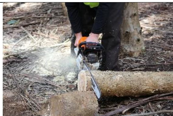
Figure 99: Recovering a sample disc from a tree stem. (Sylva Systems®.)
