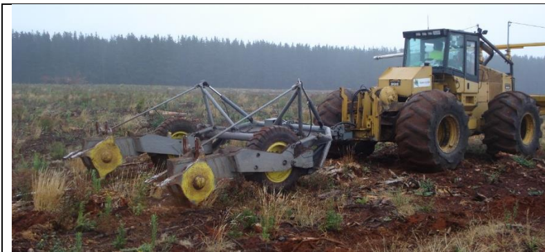
Figure 28: Second rotation site preparation with a Bräcke spot cultivator (photo by LJ Parsons ® ).
