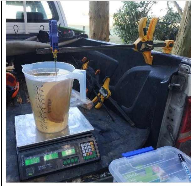
Figure 103: The scale and measuring jug setup with the overhead frame from which the samples were suspended. (Forest Quality®.)
