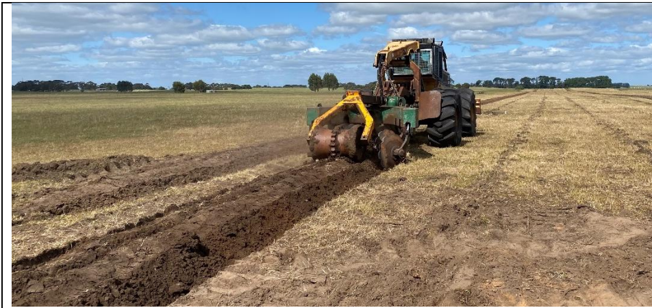
Figure 35: Mound ploughing over rip lines (photo by DJ Geddes © ).
