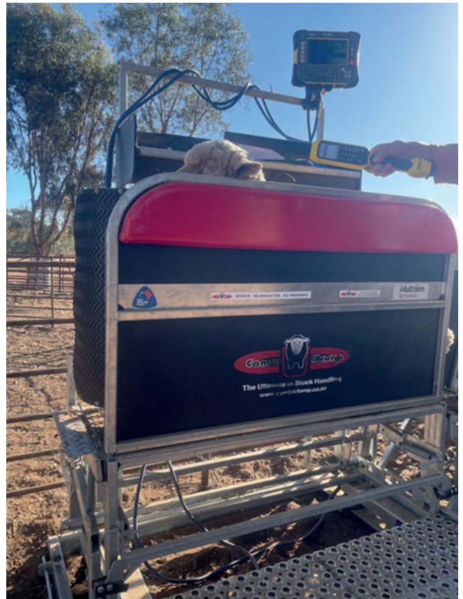
Figure 2: Combi Clamp handler and wand being used to record weight data.
