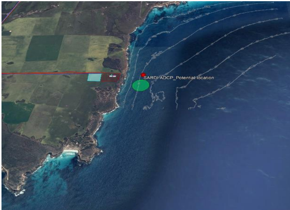
Figure 2: Image from cruise plan showing close-up of the mooring location (red circle) in relation to the proposed desalination plant site, including the region for the outfall region (green circle). Grey lines indicate bathymetric contours at 5 m intervals starting at 10 m. The oceanographic mooring is located in approximately 20 m of water.
