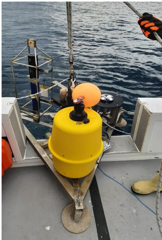
Figure 3: The oceanographic mooring being readied for deployment. An Acoustic Doppler Current Profiler (ADCP) is on the right, a Conductivity, Temperature, Depth sensor (CTD) is on the left and the (yellow) acoustic release float pack is in the front and centre.
