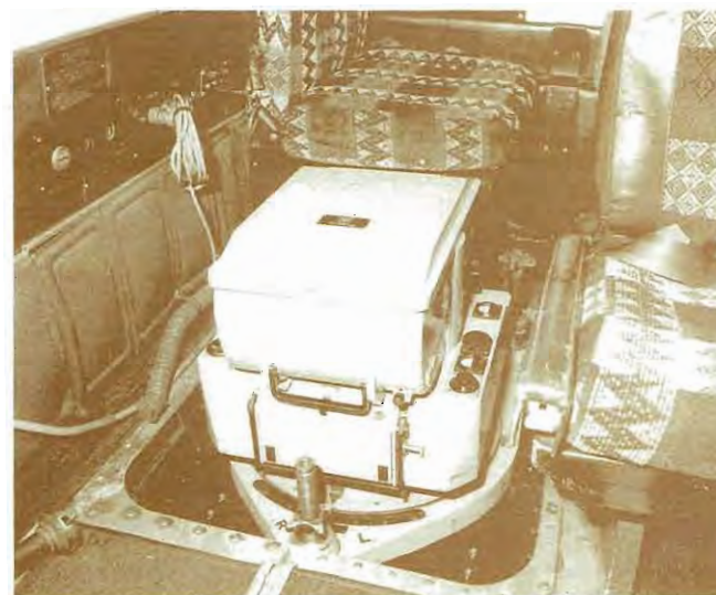
Aerial survey camera in the Department's aircraft
