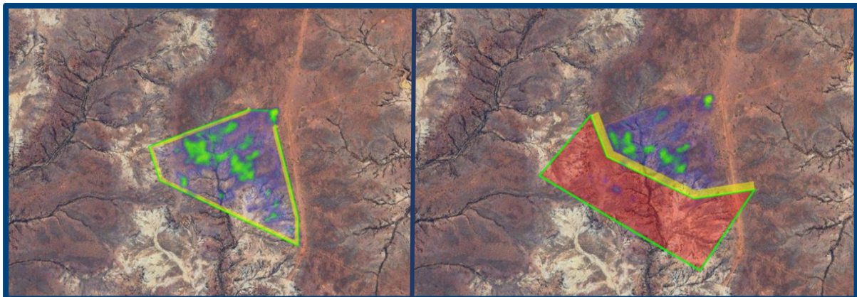
Fig. 1. The two virtual fence configurations implemented during the 7-day training period preceding trial commencement. Areas of blue and green shading represent a heat map of the GPS locations of the cattle during this time.
