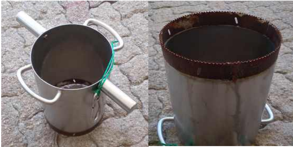
Figure 3-3: Corer used to obtain seagrass samples and shows cutting teeth on the right.
