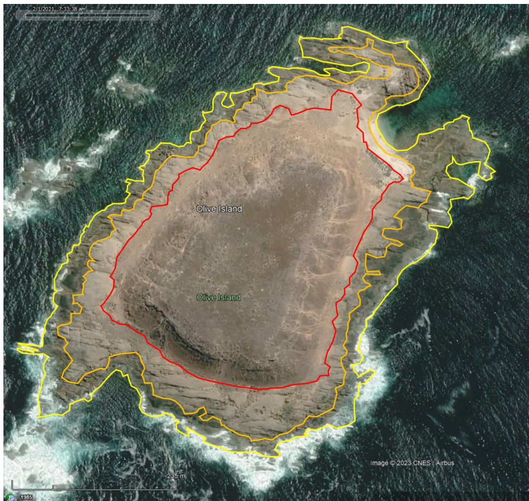
Figure 5.3 Example (using Olive Island) of the boundaries derived for area above mean-tide (yellow), area above high-tide wave-run (orange), and area above storm-driven wave-run (red), estimated using the polygon tool in Google Earth Pro.
