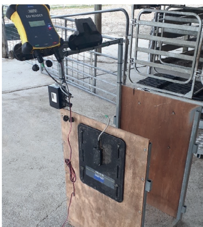
Figure 3: Portable race reader fabricated on farm incorporating a pair of panel antenna and Tru Test XRP2 eID reader. Further refinement of the design is planned to improve read rate.
