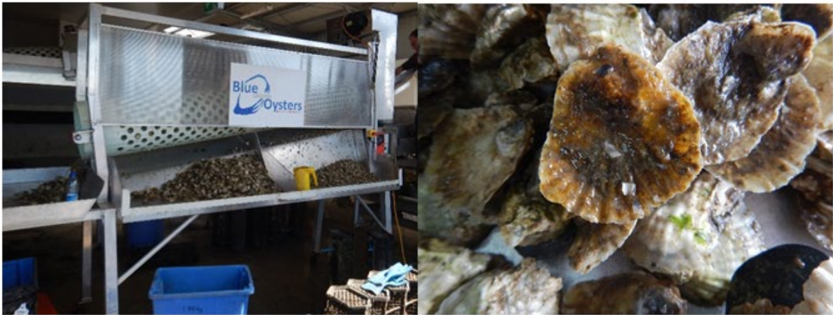
Figure 3.18 Rotating barrel grader selecting for 35 mm hole size grade (largest pile in photo) Native Oysters ( Ostrea angasi ) for grow-out trials in Blackman Bay, Dunalley, Tasmania, Australia.
