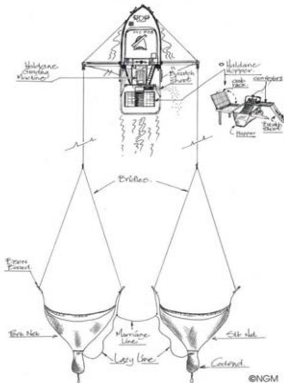
Figure 1: A double rigged trawl set used by the majority of vessels in the Gulf St Vincent Prawn Fishery.
