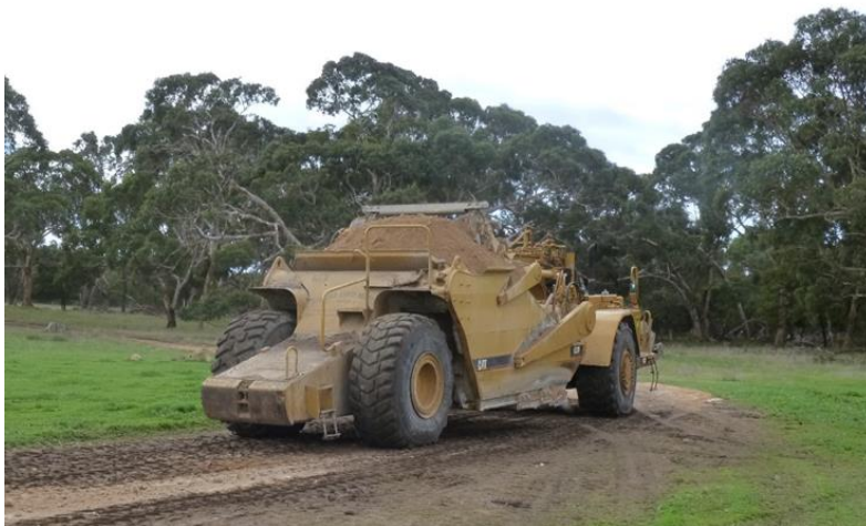
Figure 18: Using a scraper to build a log truck road using gravel recovered on the farm (Photo by DJ Geddes®)
