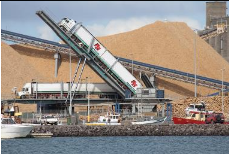
Figure 15: Unloading B-double chip trucks at one of the Portland woodchip export terminals (Photo by DJ Geddes®)
