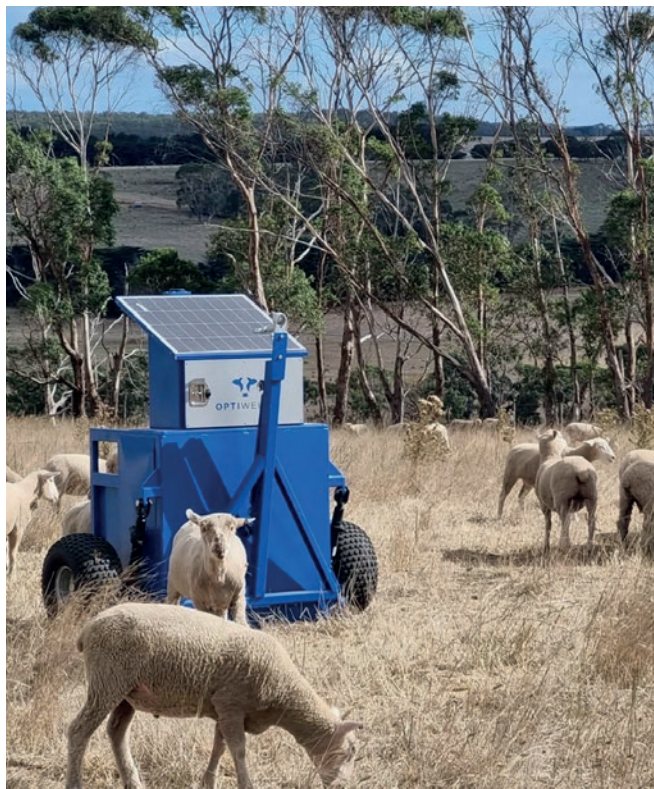
Figure 2 and 3: Optiweigh Sheep unit capturing live weight data of lambs in the paddock.
