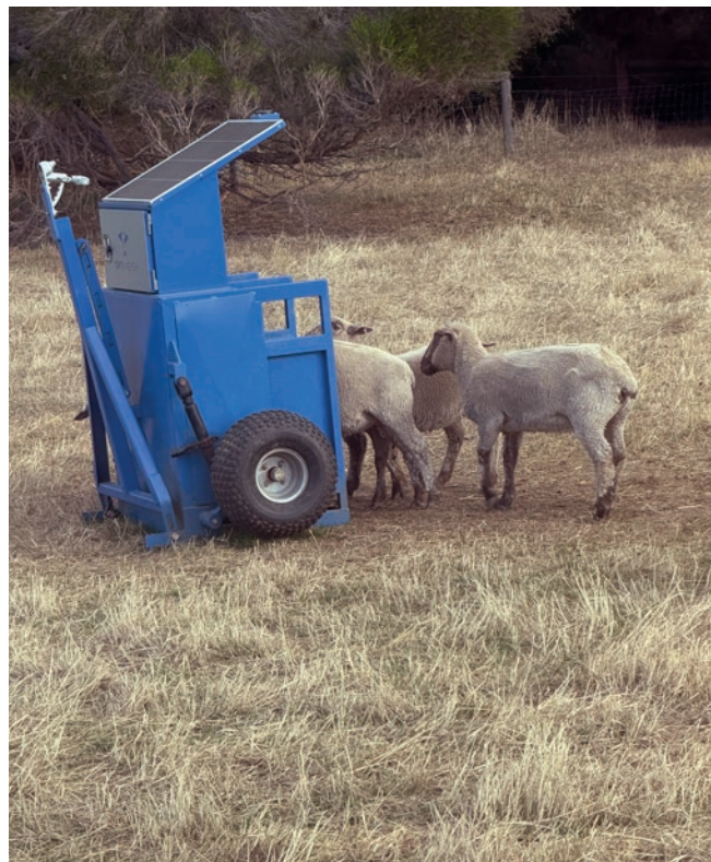
Figure 2 and 3: Optiweigh Sheep unit capturing live weight data of lambs in the paddock.
