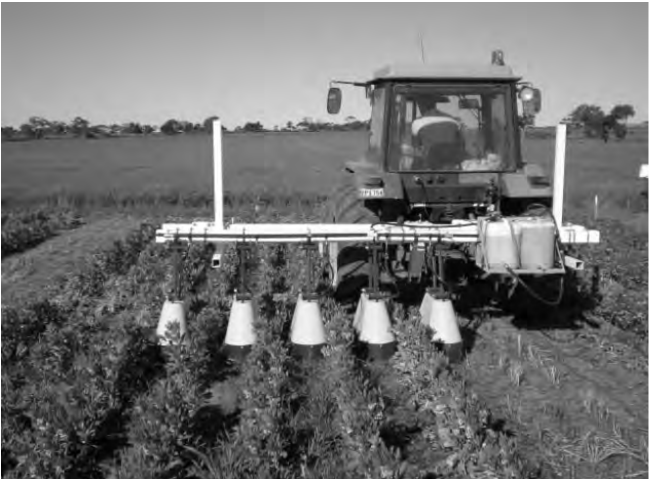
Figure 1 Commercial shields used to spray knockdown herbicides between crop rows at the experimental site.
