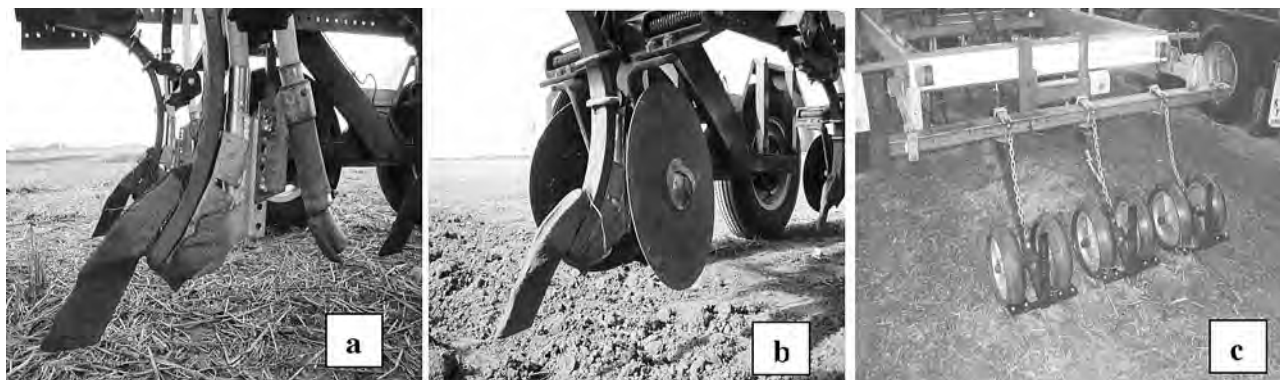
Figure 1: Knife point system used in the trial (a), with rolling shield kit closed in 125 mm (b), and 100 mm banked press wheels (c)
