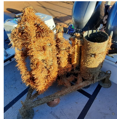
Figure 4: (Left) Location of the mooring (red cross) deployed in the western sector of the Fitzgerald Bay Aquaculture zone. (Centre) Picture of the mooring pre-deployment. (Right) Picture of the SAIMOS mooring recently recovered from upper Spencer Gulf off Point Lowly showing the extent of fouling after 6 months in the water.
