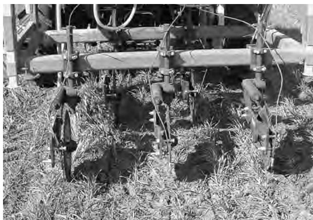
Figure 2: Disc coulters applying dissolved urea to late tillering barley at Tooligie Hill.
