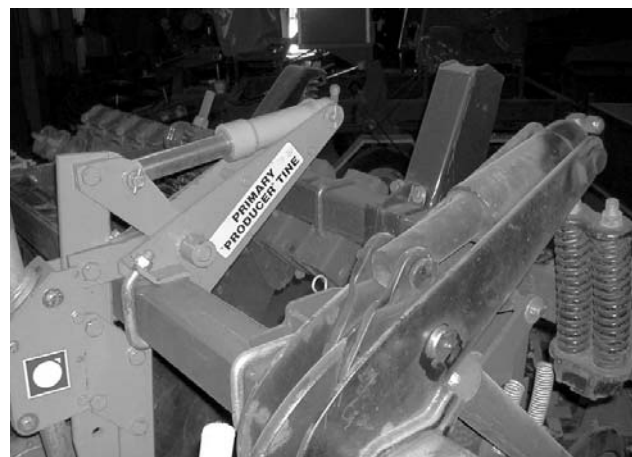
Figure 3: The ideal trip system in stony soils combines mechanical and hydraulic breakaway characteristics.
