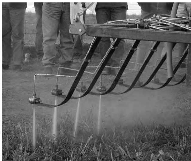
Figure 1: Root Zone Injector (RZI) demonstration with the skids raised off the ground. Note: only four jets were photographed in the firing phase, the other four are between pulses.
