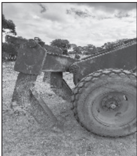
Figure 1. Delver used to implement tillage treatment on the Plozza + Delving block.
