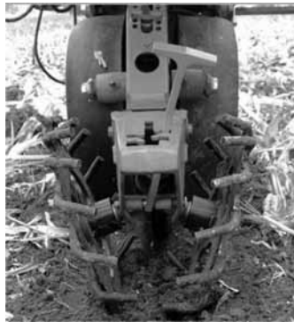
Bent finger Posi-Close planter wheels from Schlagel Manufacturing, USA, emphasizing greater furrow packing efforts
