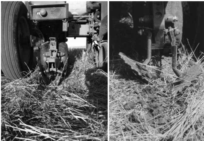
The Thompson spoked closing wheel (Exapta Solutions Inc.) on a precision planter in high residue conditions (LHS). The thin edged wheels either run parallel to travel and crumble the side walls or include 6 degree toe-out wedges to additionally gather soil over the furrow. RHS: Thompson closing wheel with Hagny high camber spoke (HCS) for improved furrow closing in low residue conditions. The HCS closing system is best used with a preceding seed firming device as it leaves the crumbled soil loose."
