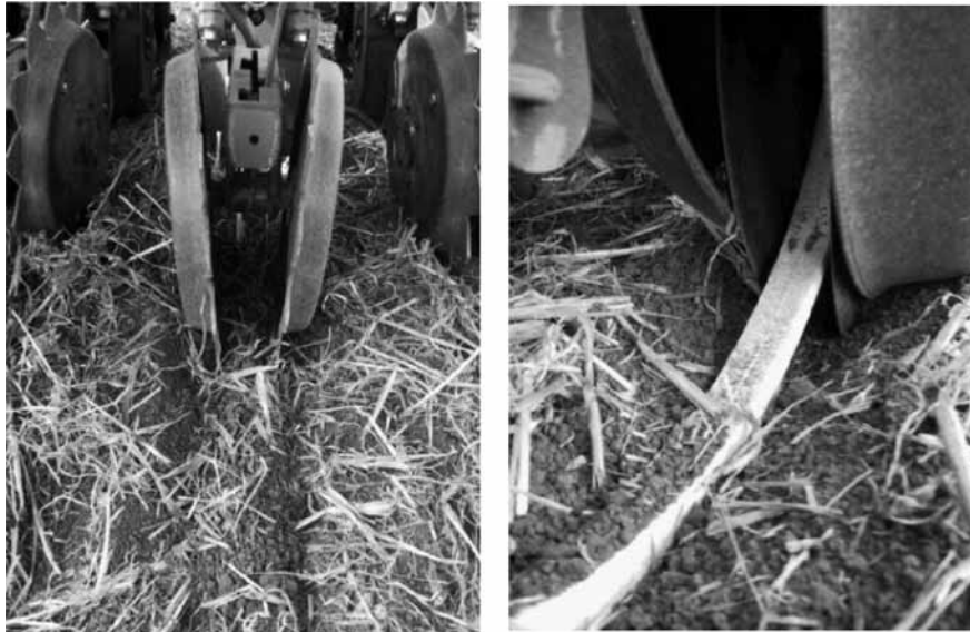
An example seed firming slide (RHS) and Furrow closing/packing wheels (LHS) on a Bertini double disc seeding opener
