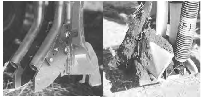
Figure 2: Example 2x2" spread paired row (left) and 6-7" spread ribbon (right) seeding technologies.
