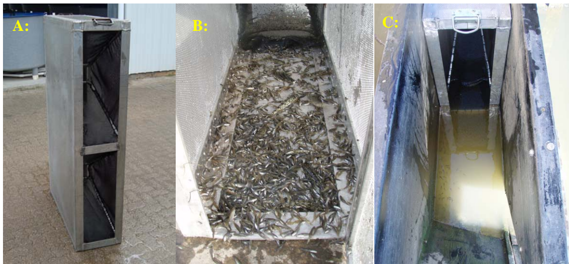
Figure 6. Entrance trap for the bottom of the fishway showing A: entrance funnels through which fish enter the fishway, B: rear door for removal of catch showing a variety of fishes from a trial run and C: The entrance trap slides flush into the bottom of the fishway without obstructing the entrance.
