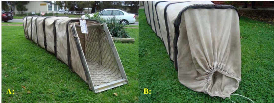
Figure 5. Exit trap for the top of the fishway showing A: attachment mechanism and B: closable cod end for removing fish catch.
