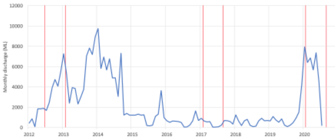
Figure 1: Monthly discharge of brine (ML) from the Adelaide desalination plant from 2012 to 2020. Red lines indicate infaunal sampling events. Source: Loo et al. (2021).
